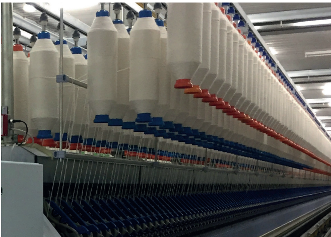
Ring spinning application driven by tangential belt
